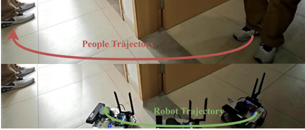
Fig. 10: Kapao [4], a real-time people-tracking application on our four-wheeled robot with a CNN-based human keypoint detection model.
